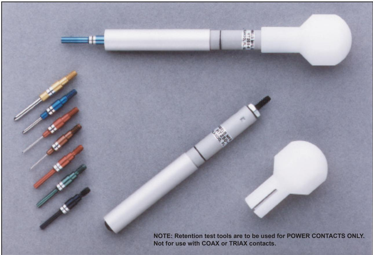
**NOTE: Retention test tools are to be used for POWER CONTACTS ONLY. Not for use with COAX or TRIAX contacts.**
